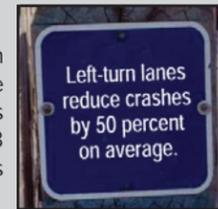
Left-turn lanes also substantially increase the capacity of many roadways. A shared left-turn and through lane has about 40 to 60 percent the capacity of a standard through lane. [4]. A synthesis of research on this topic found a 25 percent increase in capacity, on average, for roadways that added a left-turn lane. [13]
